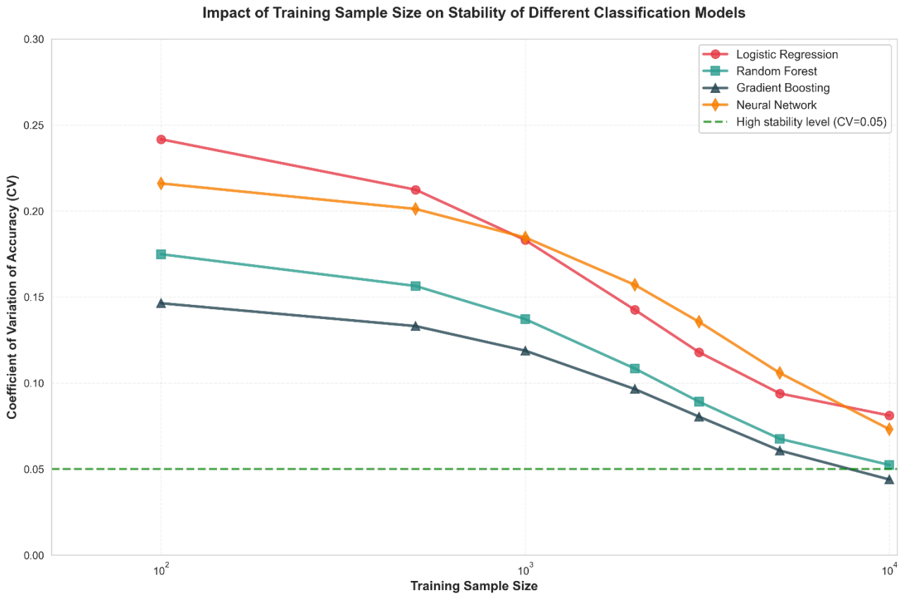
Fig. 1. Effect of training sample size on the stability of different classification models
